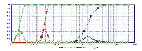
Fig. 2. Integral and differential distribution curves of ground in a roller mill and the resulting release of calcium polysulfide.
