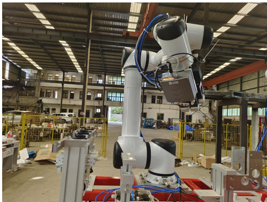
Figure 4.1 Actual picture of the designed six-degree-of-freedom robotic arm
