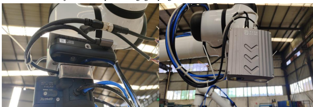
Figure 4.2 The robotic arm equipped with an arm-mounted visual sensor
